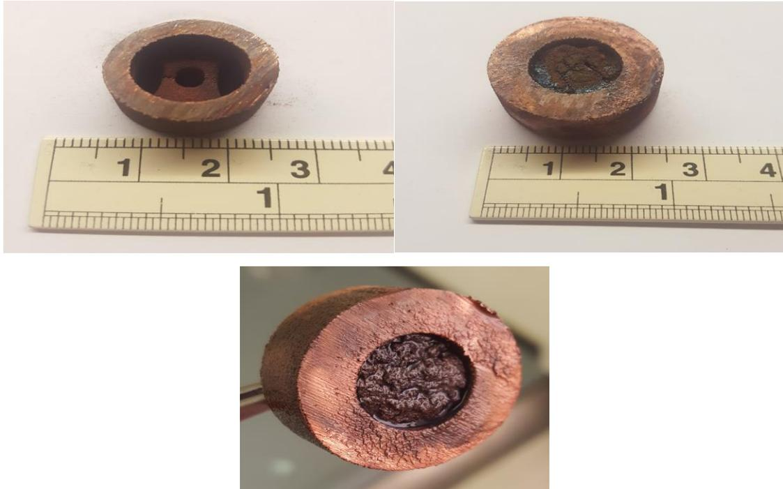
**FIG 9: SPECIMENS TREATED WITH ULTRASONIC AGITATION IN COPPER-AMMONIA COMPLEX SOLUTION. LIGHTLY SINTERED SPECIMEN TREATED FOR 6 HOURS (LEFT), AND HEAVILY SINTERED TREATED FOR 9 HOURS (RIGHT). HEAVILY SINTERED PART AFTER 8 HOURS OF TREATMENT PICTURE BOTTOM.**
