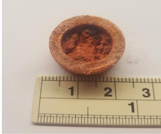
**FIG 8: LIGHTLY SINTERED SPECIMEN TREATED IN CITRINOX CLEANER FOR 6 HOURS.**
