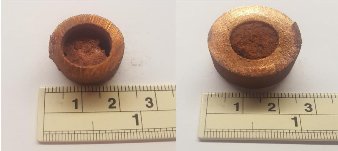
**FIG 6: SPECIMENS TREATED WITH ULTRASONIC AGITATION IN TAP WATER. LIGHTLY SINTERED POWDER TREATED FOR 6 HOURS (LEFT), AND HEAVILY SINTERED POWDER TREATED FOR 9 HOURS (RIGHT).**
